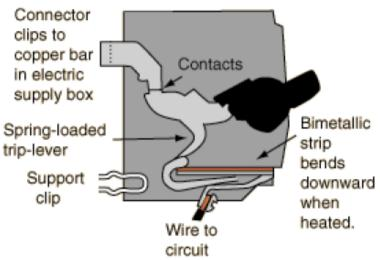
This is a simplified mechanism. the standard breaker has several springs and levers. For when you plug a toaster and an iron in the same outlet!!! .....
