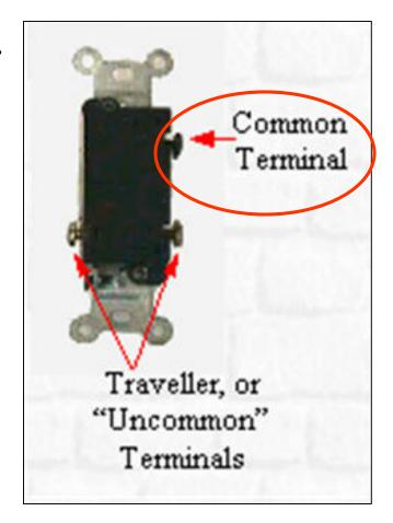
The heart of a 3-way circuit is the **3-way switch**. Unlike a common wall switch, the 3-way switch has three active terminals (plus a ground in up-to-date installations). Only one of them is important to identify for the purposes of replacement... the <u>COMMON TERMINAL</u>. Though our graphic (left) shows the common terminal in a certain position, the fact is that it could be any terminal on your individual switch.
