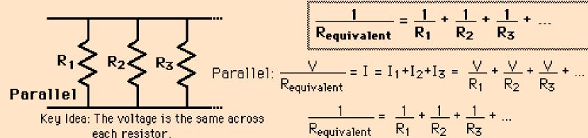
$$\frac{1}{R_{equivalent}} = \frac{1}{R_1} + \frac{1}{R_2} + \frac{1}{R_3} + \dots$$
