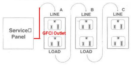
Placing the GFCI in position A will provide protection to "load side" receptacles B and C.
