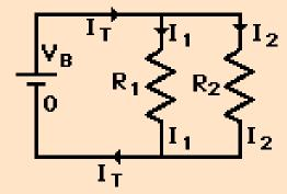
For a parallel circuit the current divides such that  $\,I_{\,T}\,=\,I_{\,1}\,+\,I_{\,2}\,$
