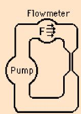
A meter for volume flowrate must be in series to measure the flow, but must not appreciably affect the flow.
