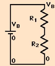
For a series combination, the sum of the voltage drops across  $R_1 \& R_2$  must sum to equal  $V_B$  .
