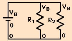
The voltages across elements in parallel are equal. This is one of the implications of the voltage law – since the change across either  $R_1$  or  $R_2$  must be equal to the battery voltage  $\mathbf{V_B}$ , then they are equal to each other.
